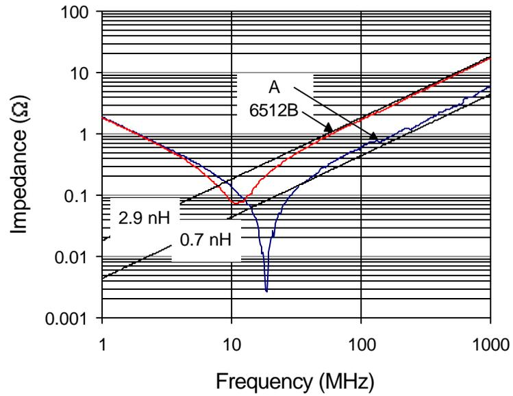
Impedance of a SMT capacitor (6512B) and a BC test board (A)
