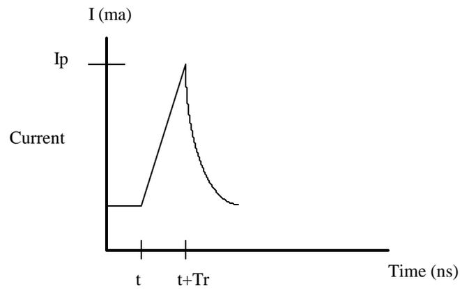
**Typical Output Switching Current Waveform
