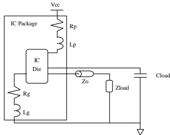
**Integrated Circuit Package and Load Model**
