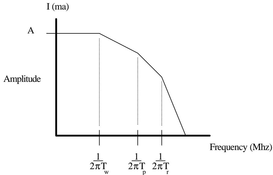
**Typical Output Switching Current Fourier Transform**
