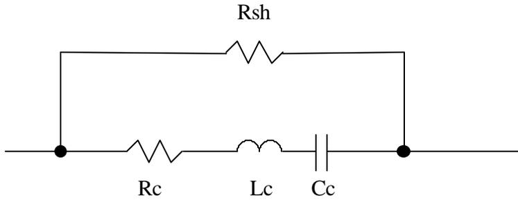
**Lumped Element Capacitor Model**
