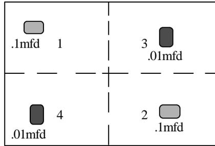
Capacitors of correct value should be added in pairs 1,2 and 3,4 in opposite quadrants of the PCB. This suggestion also applies to individual planes as split power planes or isolated islands.
