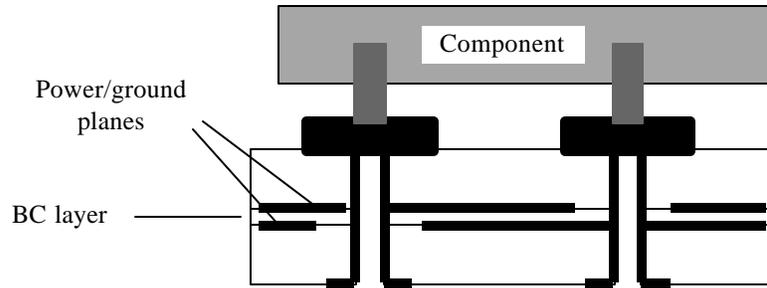
Physical model of power distribution systems using discrete capacitors vs.
