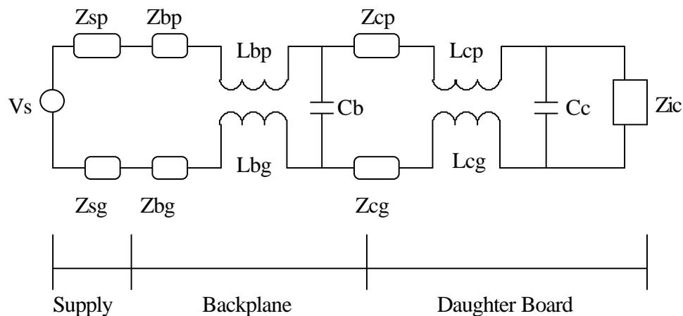
**System Level Decoupling System Model**
