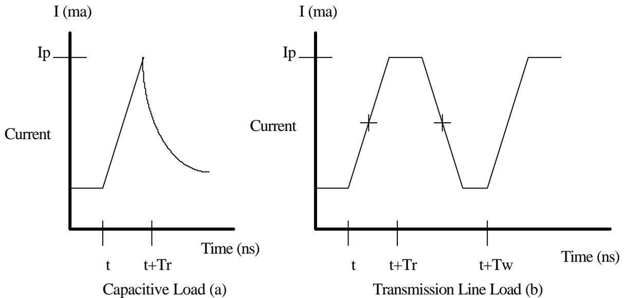
**Typical Capacitive and Transmission Line Load Current Waveforms
